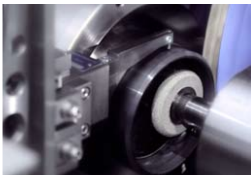
Simultaneous inner and outer diameter grinding of a silicon nitride bearing race
