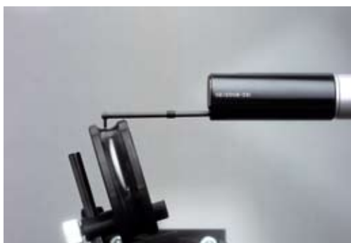
Curvature inspection of an inner raceway
